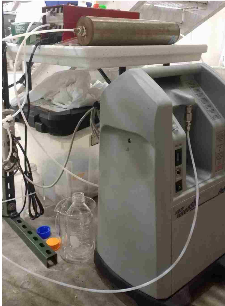
Figure 17. Ozone generator (red), oxygen dehumidifier (brown), and oxygen concentrator (grey). Oxygen from the ambient air is concentrated and it passes through an air dryer before being sent to the ozone generator to remove moisture content from the air.
