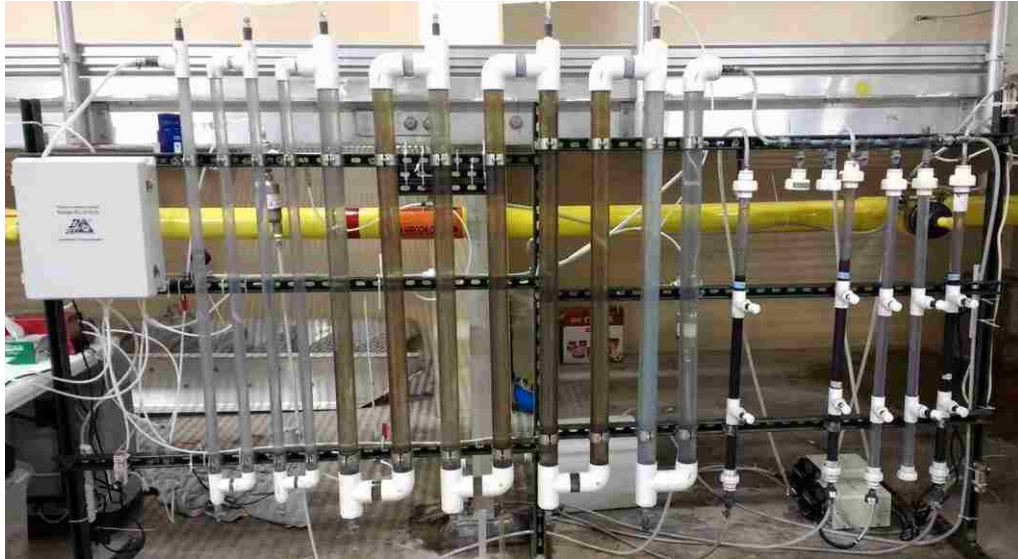
Figure 18. One liter per minute pilot-scale ozone-biofiltration system. Ozone destructor (left), ozone contactors (transparent PVC pipes), BAC column, anthracite column, and control column (left).
